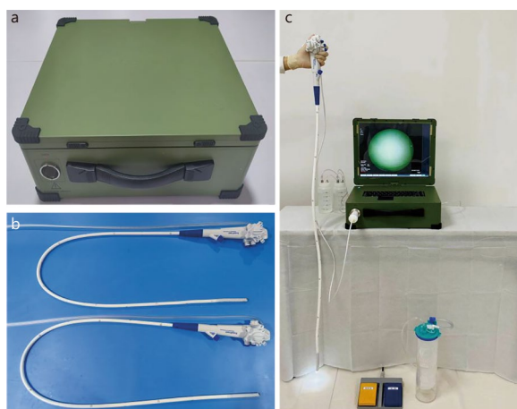
Fig. 1 The YunSendo system. a Endoscopic host. b Gastroscope (above) and colonoscope (below). c The assembled YunSendo system
